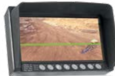
Camera setting: Horizontal line mark. This option shows a reference line on the monitor.
