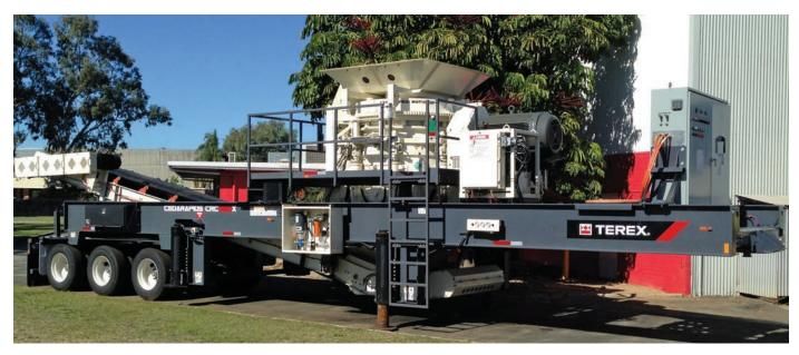
Unit shown with the following options: oversized quick release cone surge hopper and overflow chute; electrical panel; triple axle; and hydraulic run-on jacks.
