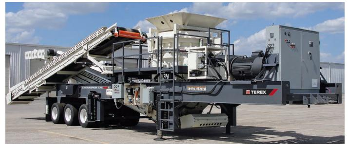
Unit shown with the following options: right-hand feed conveyor; 45' (13,716 mm) undercrusher conveyor; oversized quick release cone surge hopper and overflow chute; electrical panel; hydraulic run-on jacks; conveyor skirt boards and belt wipers.
