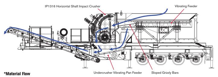
\*Unit shown with optional discharge conveyor, undercrusher vibrating pan feeder, electrical panel and hydraulic run-on jacks.
