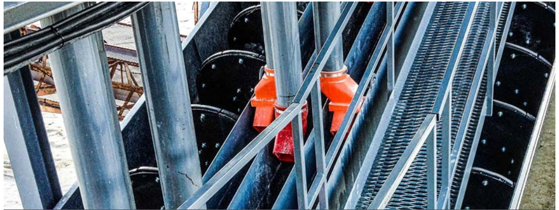
URETHANE DIRECTION DISCHARGE BOOTS WITH AR LINED FLUME
