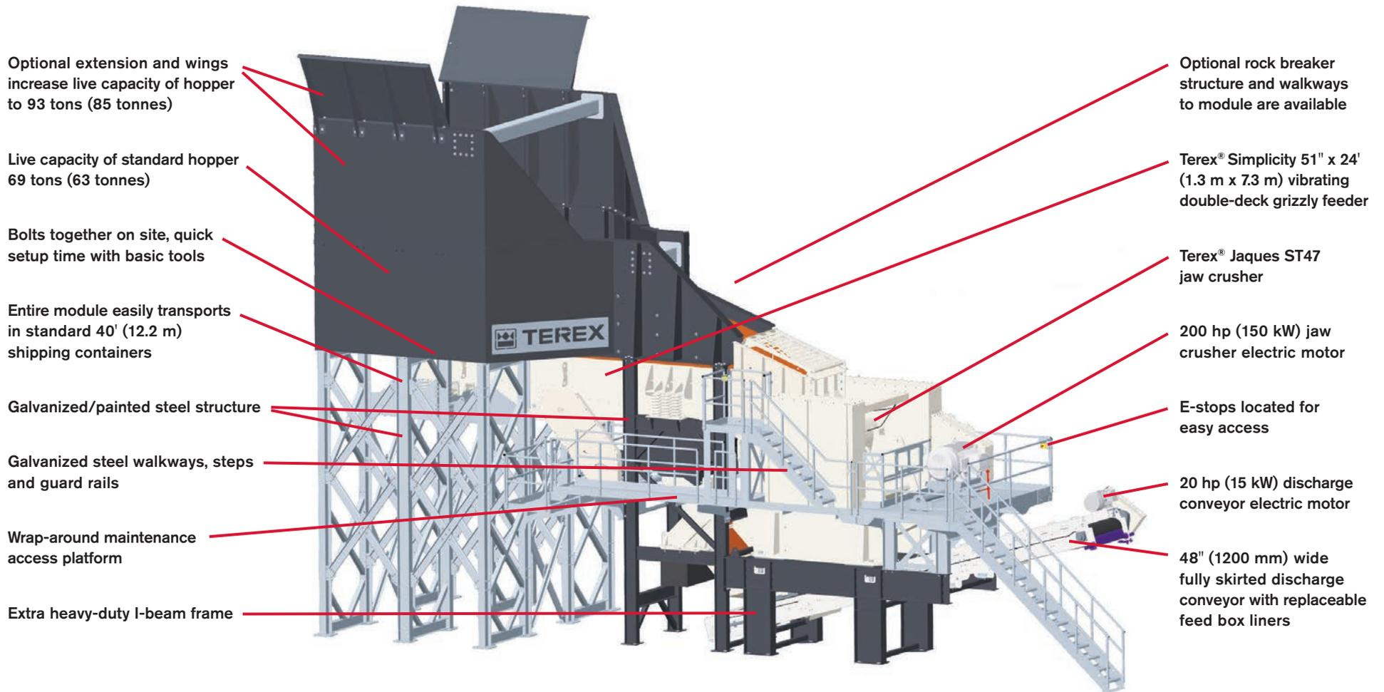
Optional extension and wings increase live capacity of hopper to 93 tons (85 tonnes)
