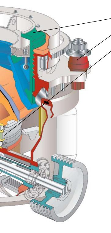
Bowl assembly with easy-change liner and brass thread inserts for trouble-free adjustments under load
