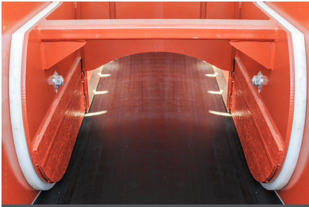
ADJUSTABLE FLOW GATE CONTROLS RATES
