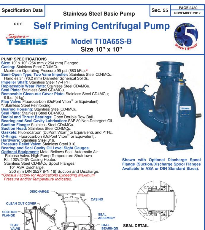
Mechanical, Oil-Lubricated, Double Floating, Self-Aligning. Silicon Carbide Rotating and Stationary Faces. Stainless Steel 316 Stationary Seat. Fluorocarbon Elastomers (DuPont Viton<sup>®</sup> or Equivalent). Stainless Steel 18-8 Cage and Spring. Maximum Temperature of Liquid Pumped, 160°F (71°C).\*
