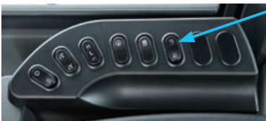
Remote positioner switch Boom / Bucket
