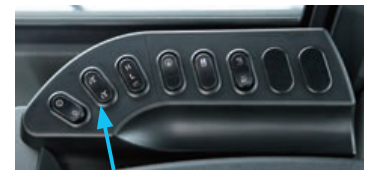
Dual mode engine power selection switch
