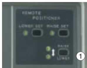
1: Remote boom positioner switch
