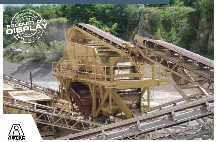
Developed based on extensive side-by-side testing of traditional and horizontal screens, KPI-JCI's Combo® Screen is known for delivering unsurpassed capacity and efficiency, while increasing feed production by as much as 25%.
