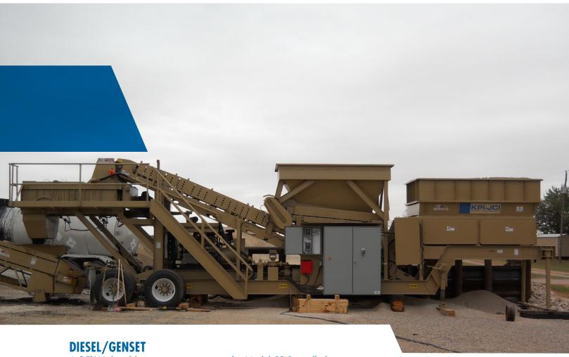
A 95kW diesel/genset is an option on the Model 52 Pugmill plants to provide self-contained power. The genset will power all on-plant functions, as well as an auxiliary silo.
