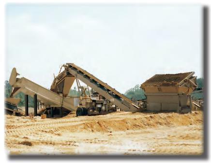
The 271K offers a traditional screening plant in single, double and triple deck configurations depending on plant and screen model. Capable of processing sand & gravel, topsoil, slag, crushed stone and recycled materials, these plants are a simple-to-use and highly reliable screening plant. Diesel power engine is water-cooled and powers all plant functions, as well as off-plant stacking conveyors. All plants provide easy access to the hydraulic plant controls and screen angle adjustment.
