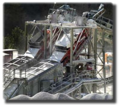
Astec Mobile Screens offers the PEP 6' x 12' series of Duo-Vibe® high frequency screens. These screens provide the material producer with a scalper top deck and high frequency bottom deck for pre-screening and/or fines removal applications. Various configurations for the screens are available in both portable & stationary structures, as well as mobile screening plants depending on model.
