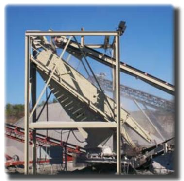
Astec Mobile Screens offers the PEP 6' x 18' series of Vari-Vibe® high frequency screens in single, double and triple deck screen configurations in stationary applications. Other configurations are available in portable structures, as well as mobile screening plants depending on model.
