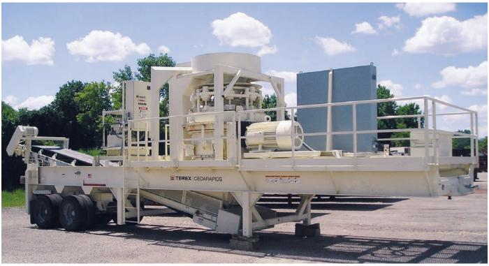
Note: The overflow chute and hopper support structure shown in the above photo are not included with a standard plant.
