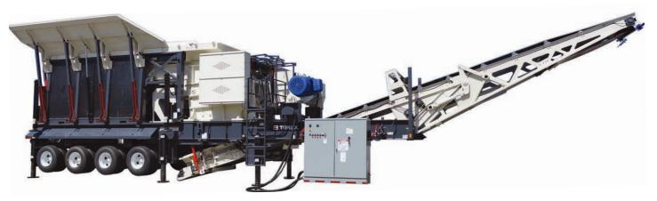
Note: Unit shown with optional electrical switchgear panel and hydraulic lift system, extended length undercrusher conveyor with hydraulic fold, truck dump hopper with hydraulic extensions, hydraulic feeder module lift system, and hydraulic leveling/run-on jacks.
