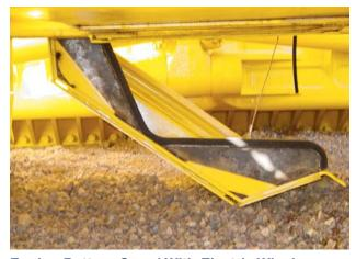
**Engine Bottom Guard With Electric Winch**
