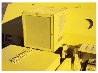
**Rear Mounted Hydraulic Cooler and Fan**
