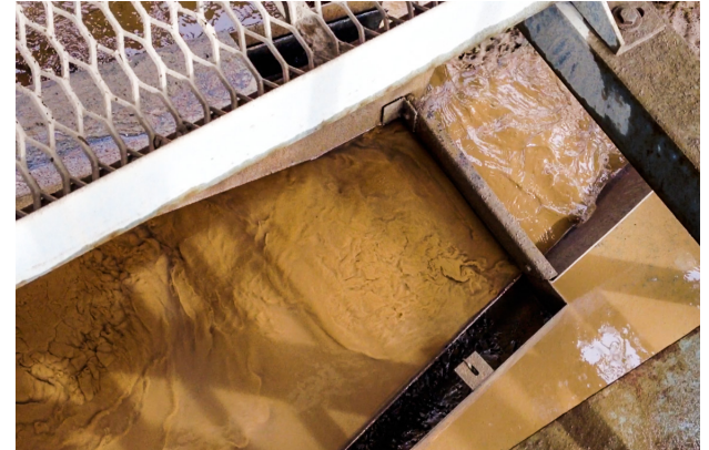
LOAD ZONE BAFFLE SETTLES FINES
