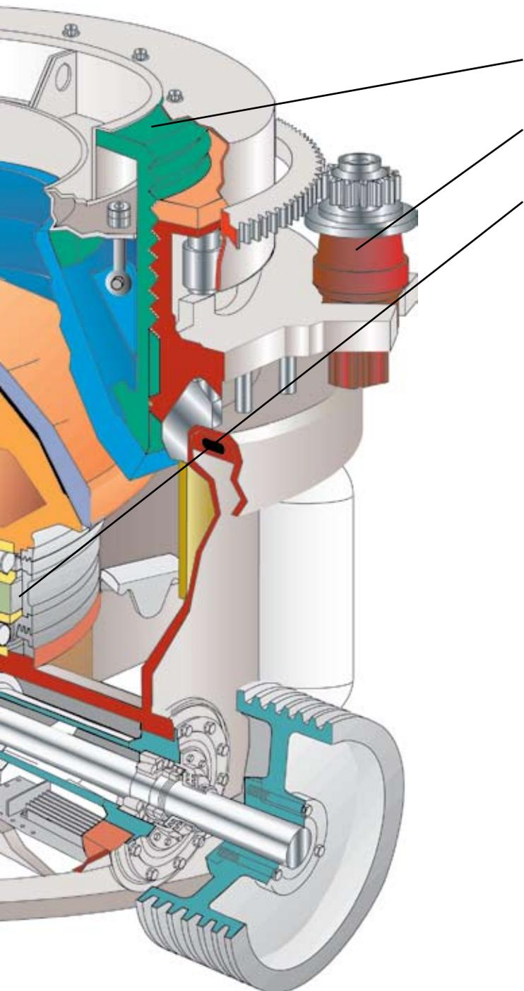
Bowl assembly with easy-change liner and brass thread inserts for trouble-free adjustments under load
