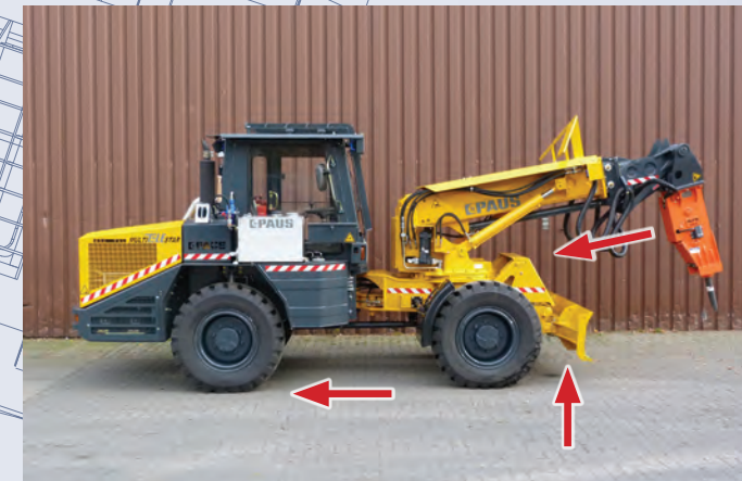
Emergency escape mode: The telescope and dozer blade are retracted automatically and reverse movement is started
