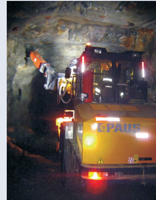
Roof damage is prevented with sensitive scaling providing sensitive and strong impact pulse, thereby improving roof safety.
