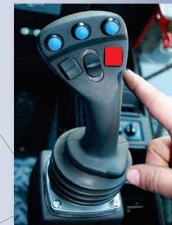
Emergency escape mode: The telescope and dozer blade are retracted automatically and reverse movement is started
