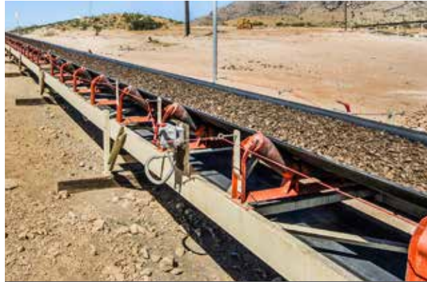
CHANNEL FRAME CONVEYOR
