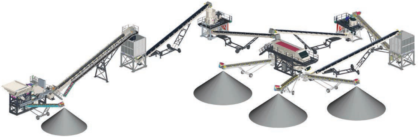
System 300 3-Stage Modular Plant (Jaw-Cone-Horizontal Screen-Cone)
