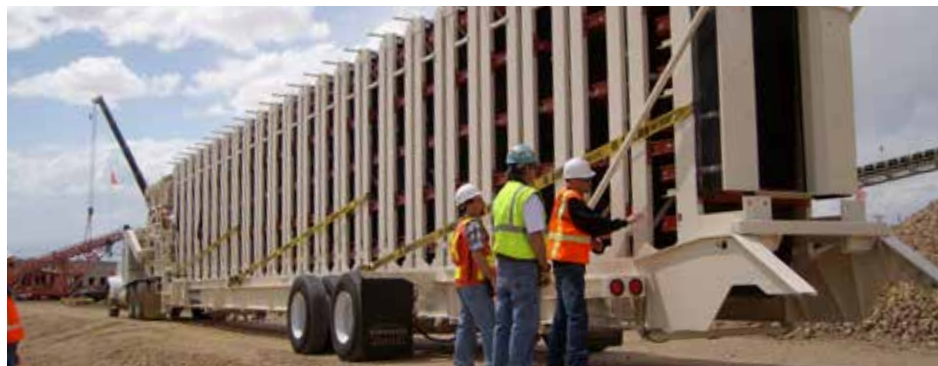
500-FEET (152m) FOLDS INTO 85-FOOT (26m) TRANSPORT LOAD
