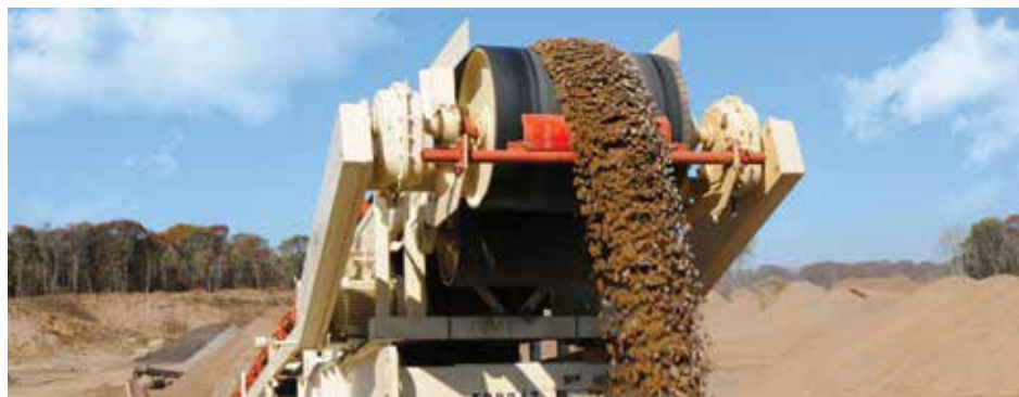
A 48-INCH (1,219mm) MODEL CAN MOVE UP TO 2,000 TPH
