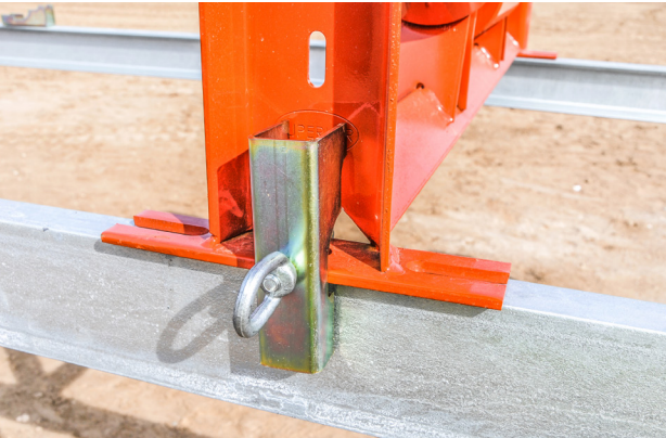
TOOLLESS IDLER INSTALLATION
