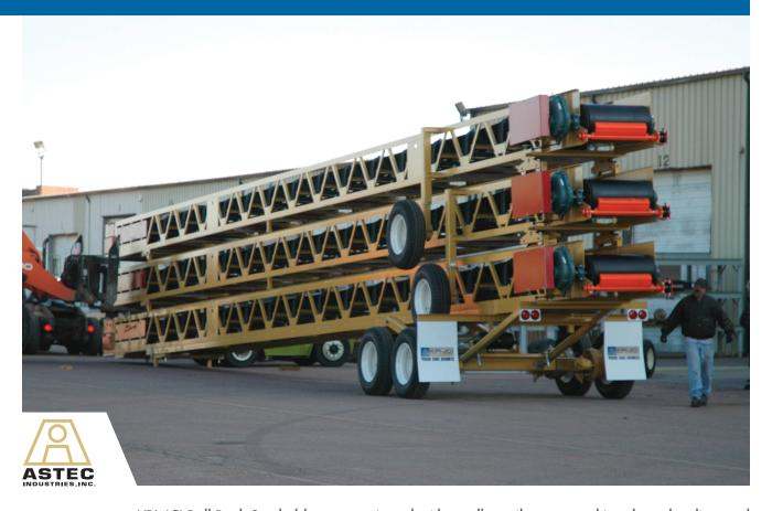
KPI-JCI Roll Pack Stackables are equipped with a roller rail system making the unloading and set-up process happen in minutes. Not only do the conveyors unload in minutes, but they load and are road-ready just as quickly and easily. The Roll Packs are available in up to 70-foot lengths, providing up to 210' of transfer conveyors on one highly portable load.
