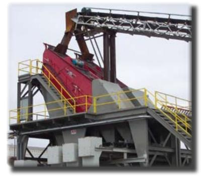
Astec Mobile Screens offers the PEP 6' x 18' series of Duo-Vibe® high frequency screens. These screens provide the material producer with a scalper top deck and high frequency bottom deck for pre-screening and/or fines removal applications. Various configurations for the screens are available in both portable & stationary structures, as well as mobile screening plants depending on model.
