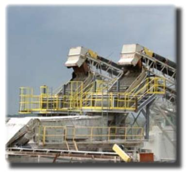
Astec Mobile Screens offers the PEP 6' x 12' series of Vari-Vibe® high frequency screens in single, double and triple deck screen configurations in stationary applications. Other configurations are available in portable structures, as well as mobile screening plants depending on model.
